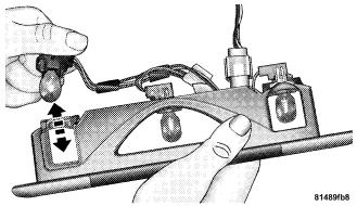
5. Pull desired bulb straight from the socket.
